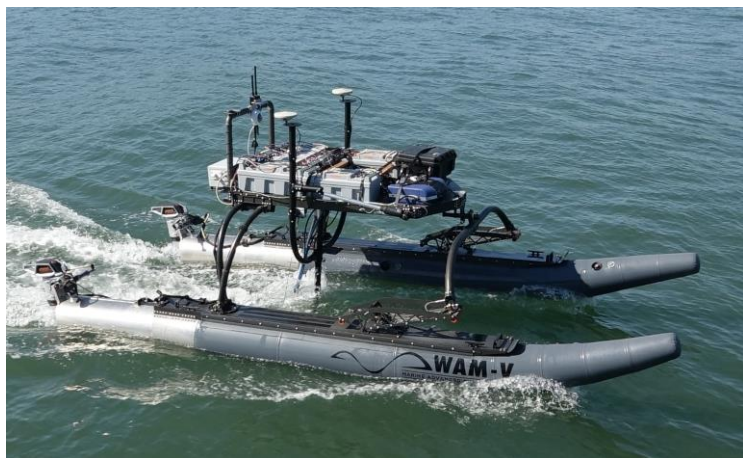
WAM-V 16 ASV with multi-beam sonar system
